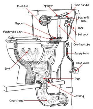
These leaks are more difficult to detect since there is usually no visible sign of water flowing down the drain. If the toilet plunger ball or flap valve does not seal properly, water slowly flows from the toilet tank into the bowl and into the drain.
