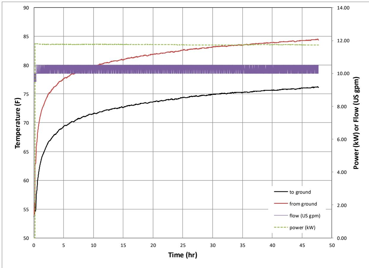
**Figure 3** Temperature, power input, and flow rate versus time data from T/C test on borehole.
