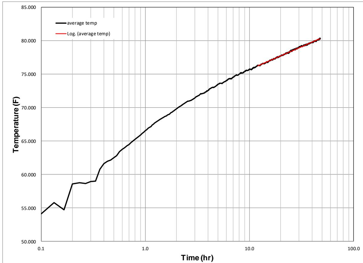
**Figure 4 Average temperature versus logarithm of time**
