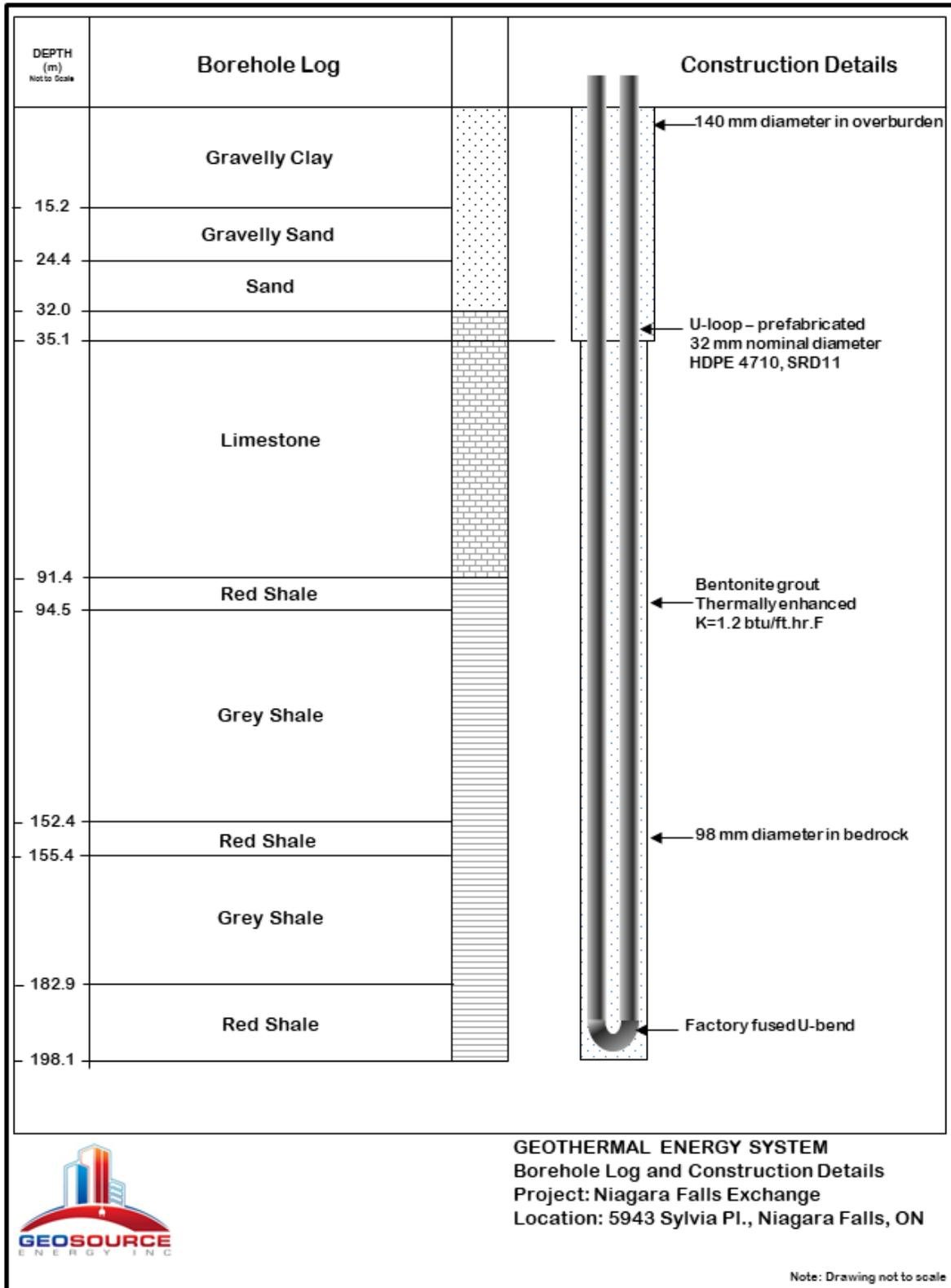
Figure 1. Borehole Log
