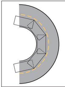
**FIGURE 3:** Cutting and overlapping GlasGrid around a curve
