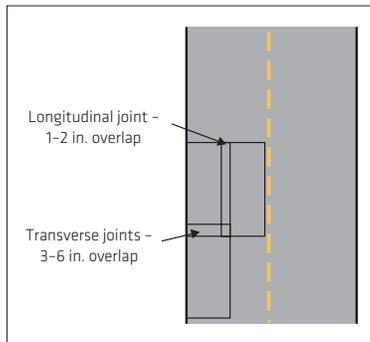
**FIGURE 4:** Overlapping GlasGrid across transverse or longitudinal joint
