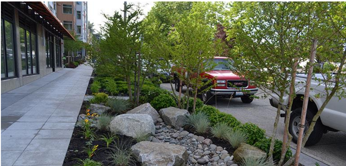
Example of bioswale incorporated within a development. Bioswales can be used to filter rainwater on-site (Image Source: City of Seattle).
