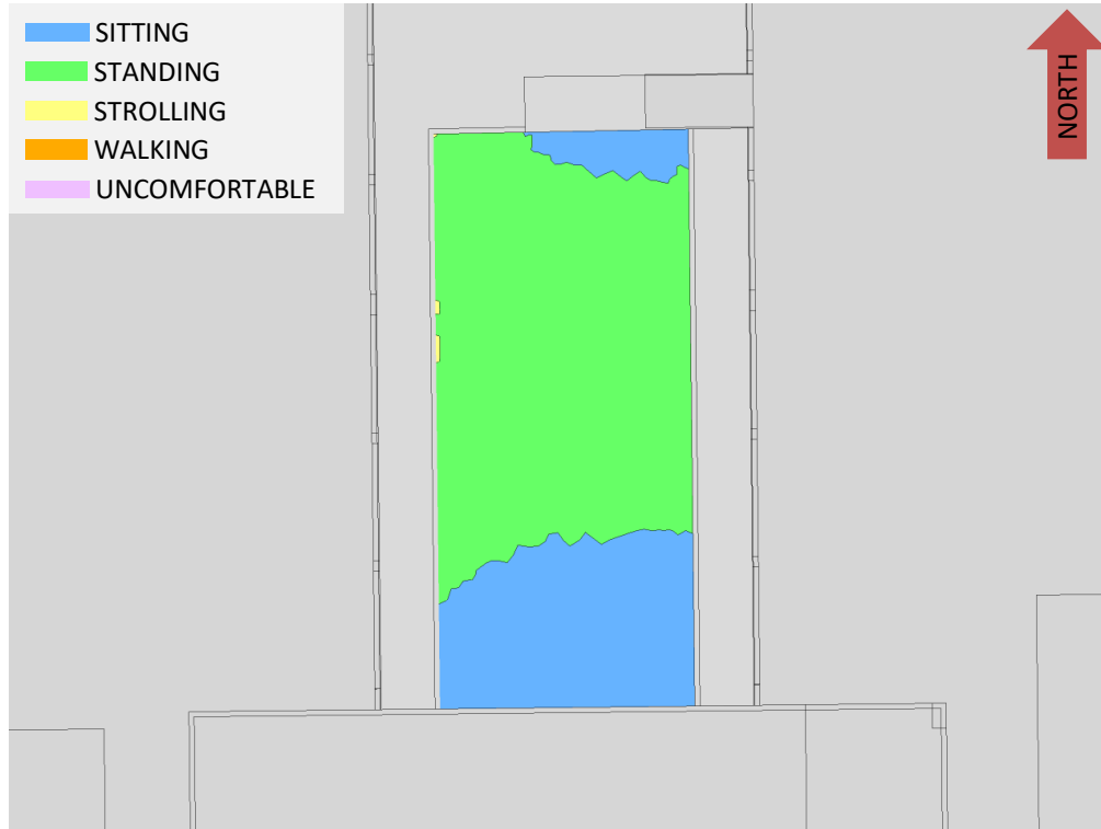
FIGURE 8A: TYPICAL USE PERIOD – WIND COMFORT, LEVEL 8 COMMON AMENITY TERRACE
