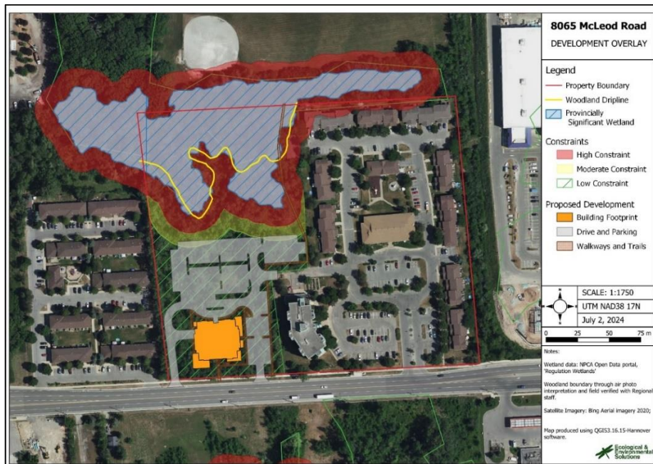
Figure 2. Natural Heritage Constraints Map with proposed development overlay (prepared by Ecological and Environmental Solutions).
