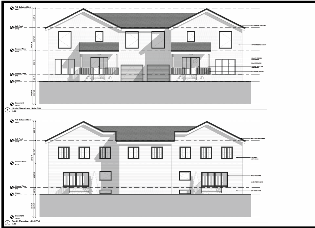
Figure 10 – Front and Rear Elevation of Semi-Detached Dwelling
