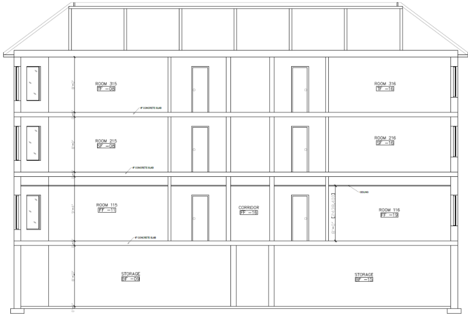
Figure 6: Cross section - South façade (Benan Hanoudi Architect)
