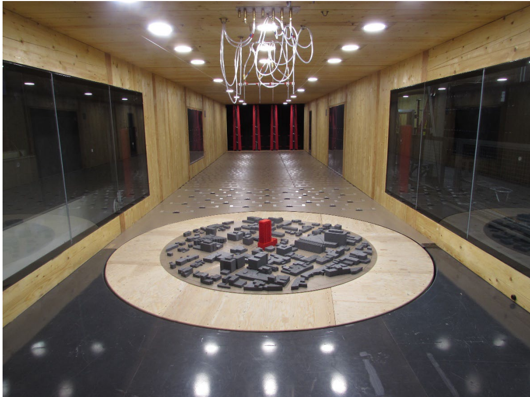
Image 5: Example Study Model in a Boundary-Layer Wind Tunnel
