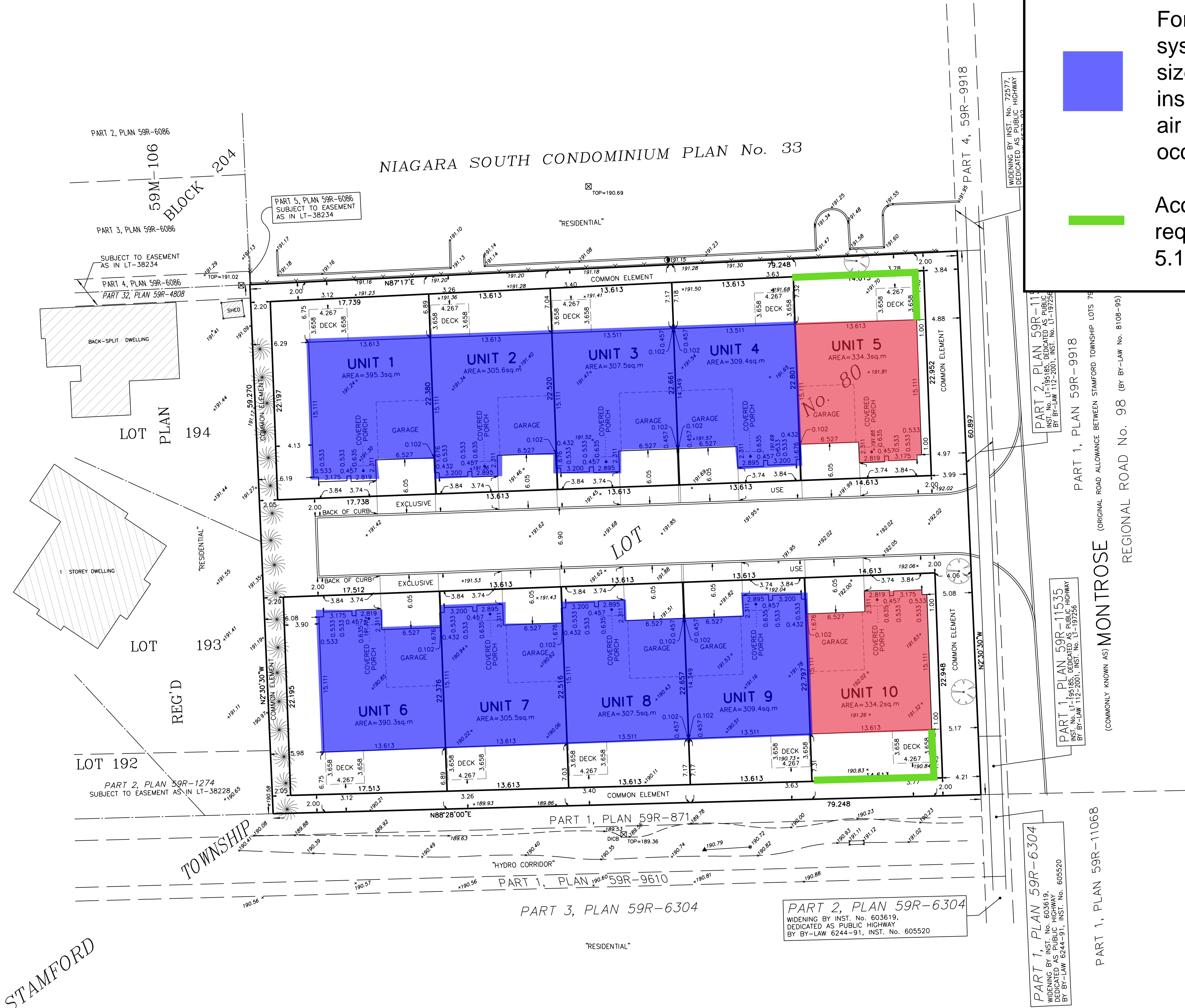
Figure 3: Draft Plan Showing Ventilation and Barrier Requirements
