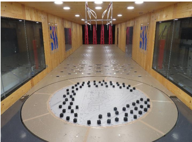
Image 2A: Wind Tunnel Study Model - Existing Configuration
