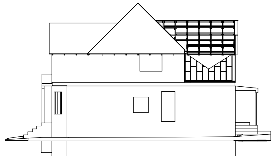
Left side view New roof and wall framing
