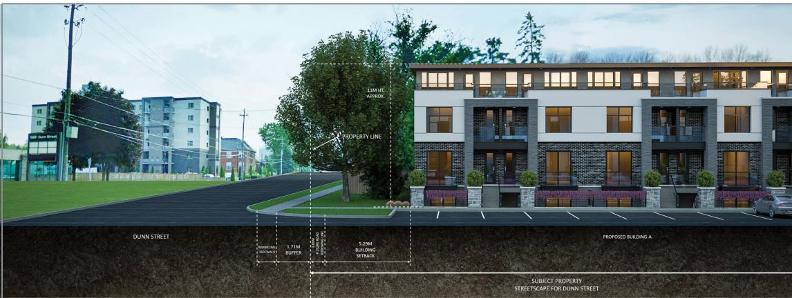
Figure 21: Proposed cross-section along Dunn Street
