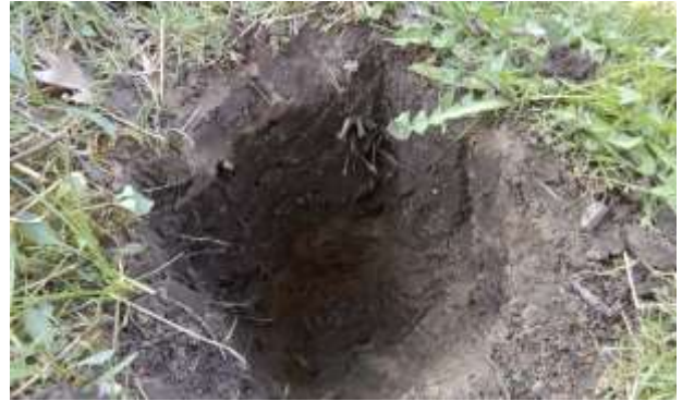
Photo 8: Sample test pit in grass area with no overburden
