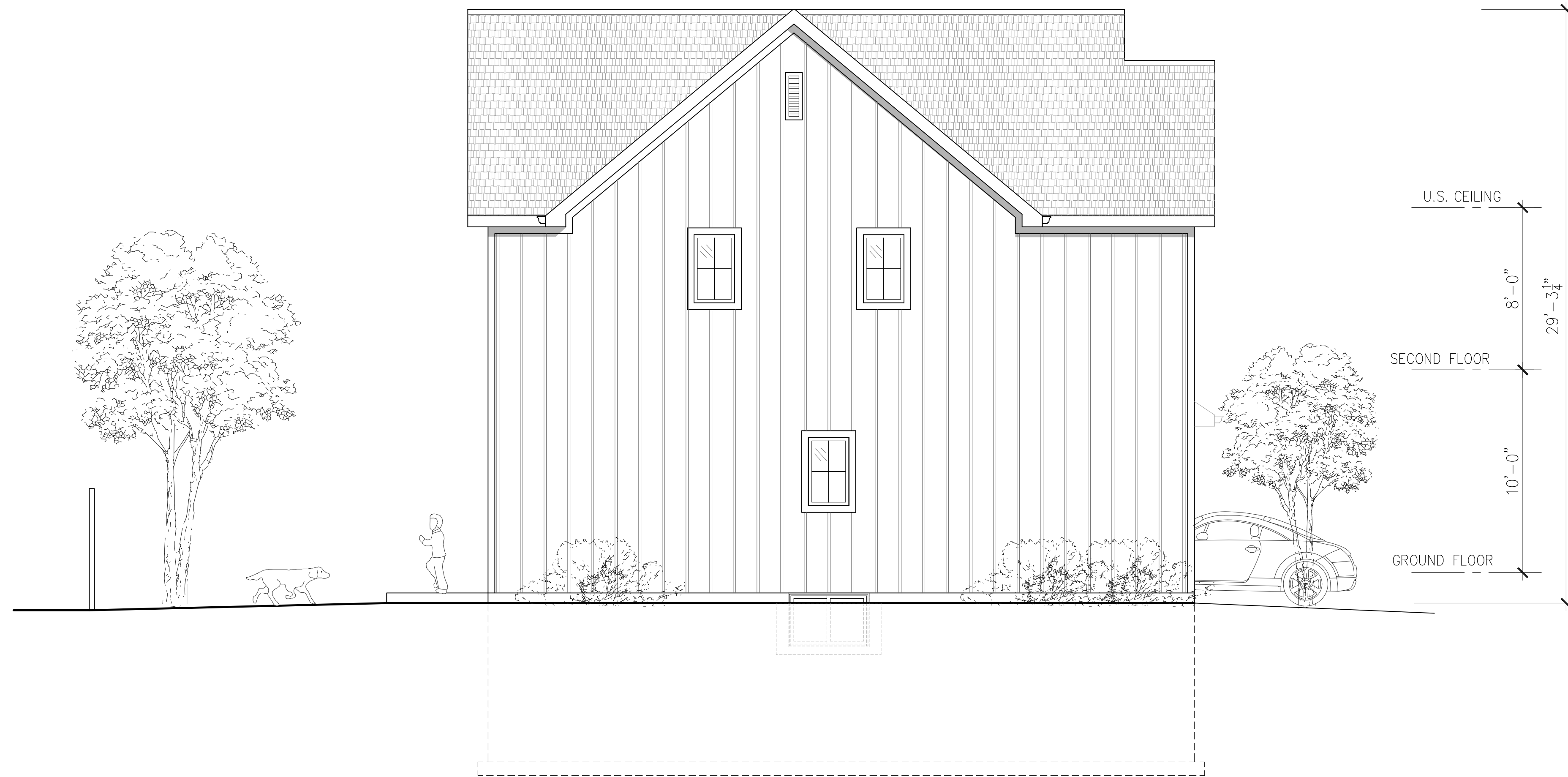
1 EAST ELEVATION - UNIT 12 (BLOCK C) SCALE: 1/4"=1'-0"
