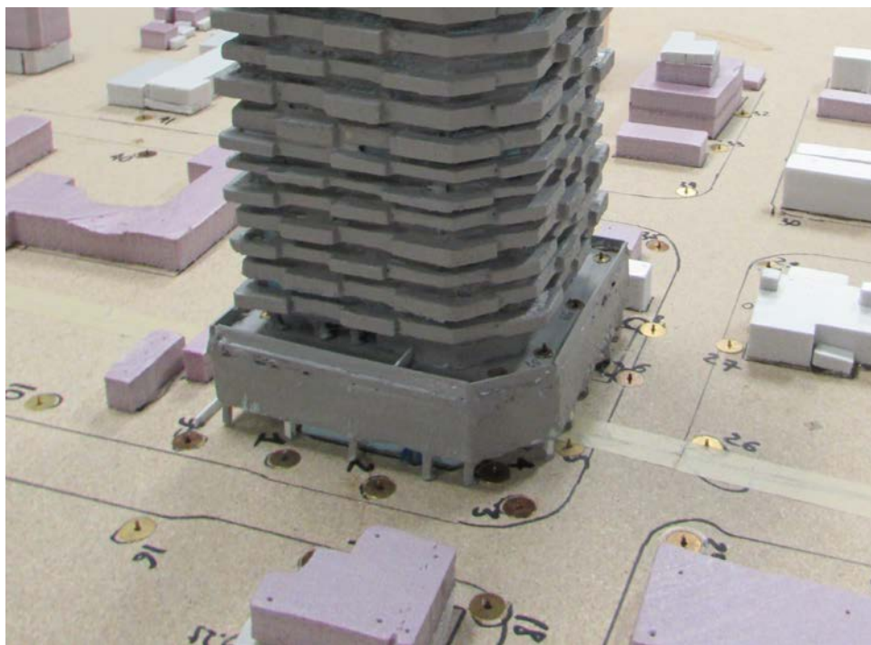
FIGURE 5a CLOSE UP VIEWS OF THE PEDESTRIAN LEVEL WIND SPEED MODELS AND CONFIGURATIONS TESTED
