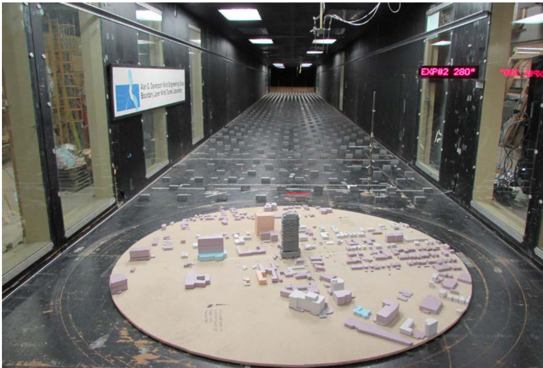
FIGURE 6 PHOTOGRAPHS OF THE MODEL IN THE WIND TUNNEL SHOWING THE UPSTREAM TERRAIN MODELS (EXPOSURES) USED
