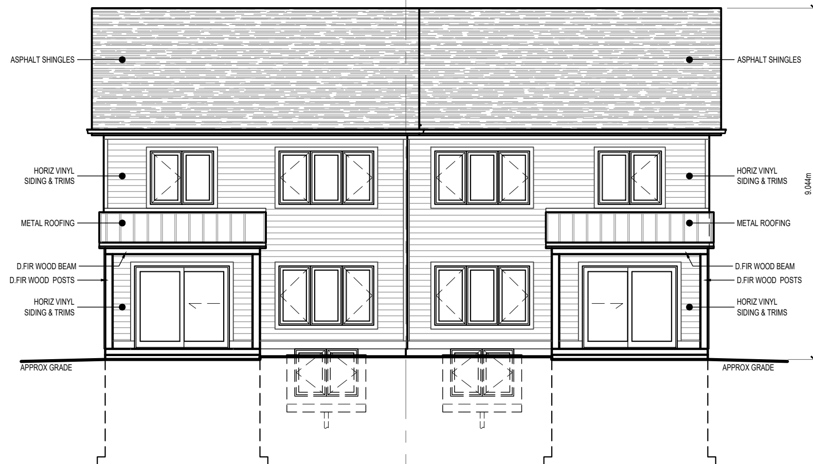
REAR / SOUTH STREET ELEVATION
