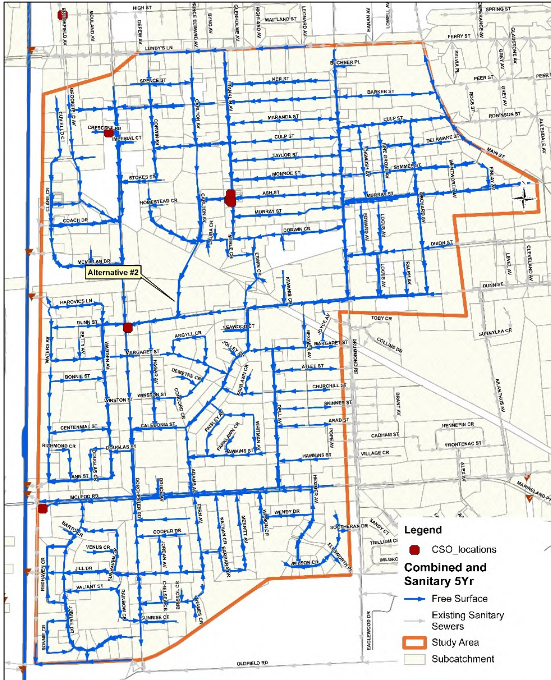
Figure 8-2: Summary of 1981 Typical Storm on Combined and Sanitary Sewer System
