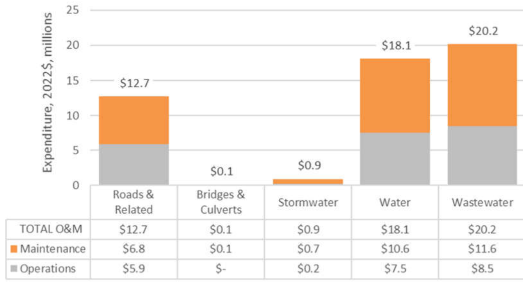
Figure 5-7 Operations & Maintenance Needs for Core Assets, by Service
